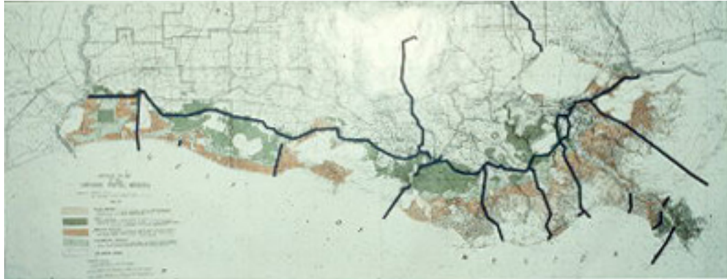
GIWW as it crosses Louisiana. Note the vertical channels added to create inland ports. The green zones are freshwater marshes, so you can see how the channels allowed salt water to decimate that type of habitat.
