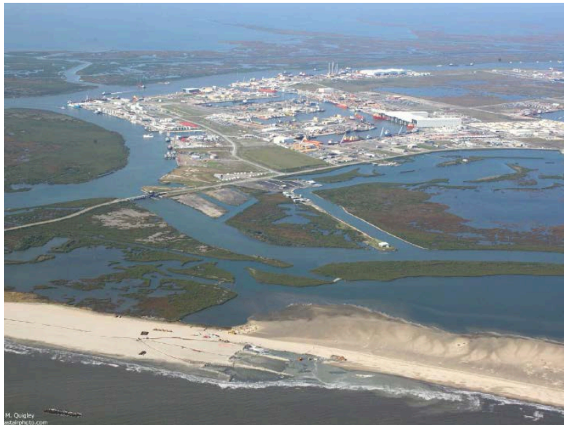
Port Fourchon in the rear, and note the pipeline in the center of the beach to the left that forks to three pipes that deliver the sand. Note how wide the beach is to the left as opposed to the right where it has progressively moved north into the estuary.
