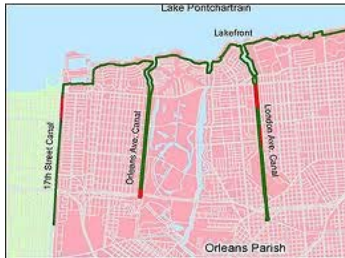
The canals with red marks where the levees broke, or, in the case of the Orleans Canal, where the water flowed through the uncompleted I-wall levee. Source unknown.
